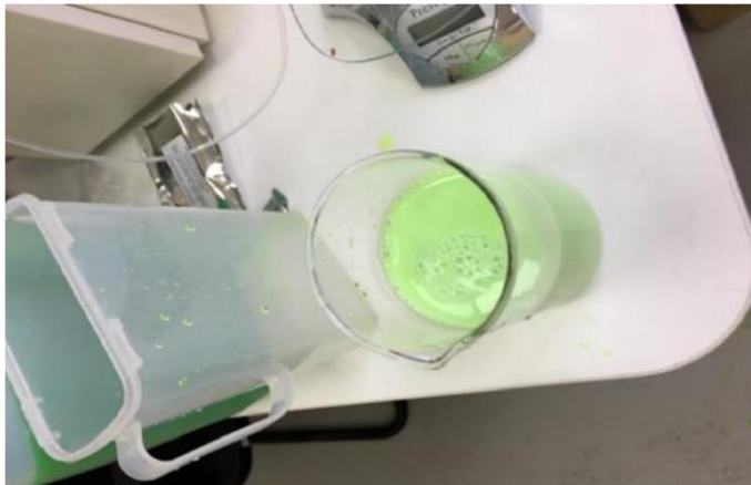
Fig.7: illustration of nanofluid with some distilled water droplets \text{Al}_2\text{O}_3 -zno using nanyl glycol nanofluid
