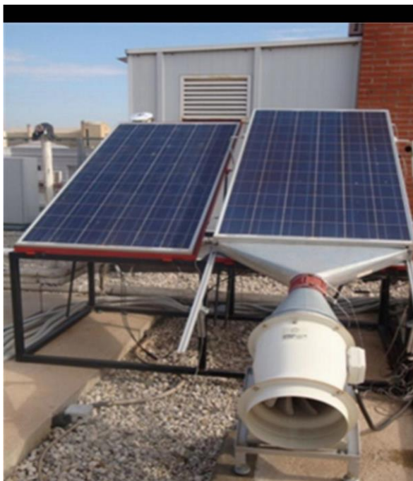
Fig. 3: illustration of the pv cell cooling system by using forced air [27]
